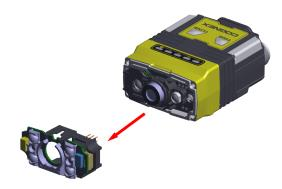
3. Unscrew the two M2x5mm Phillips head screws, remove the 6.2 mm lens mount and the 6.2 mm lens.
