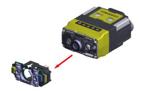
3. Turn the lens cap to the 105 mm position.
