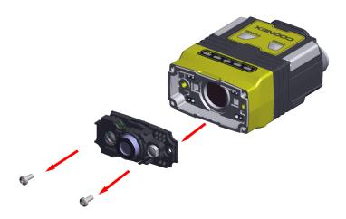
4. Place the C-Mount adapter on the front of the device, and tighten the screws.
