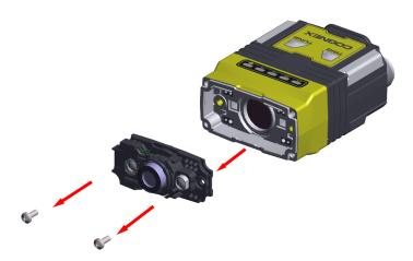
4. Attach the 16 mm lens mount and lens, and screw in the two M2x5mm Phillips head screws. Focus, if necessary. For more information, see <u>Setting Focus on page 36</u>.
