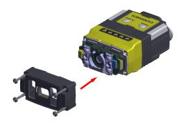
(i) Note: The rib in the front cover must be oriented to the top side.
