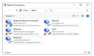
6. Right-click on the virtual adapter and select Properties. Assign a fixed IP to the network adapter starting with 192.168.111.
