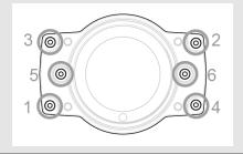
5. Place the lens cover adapter plate on the C-Mount adapter, and tighten the screws.
